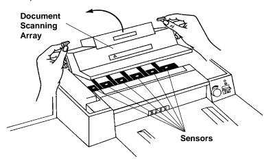
2. Tilt the Document Scanning Array toward the back of the machine, using the release handles, as shown.
